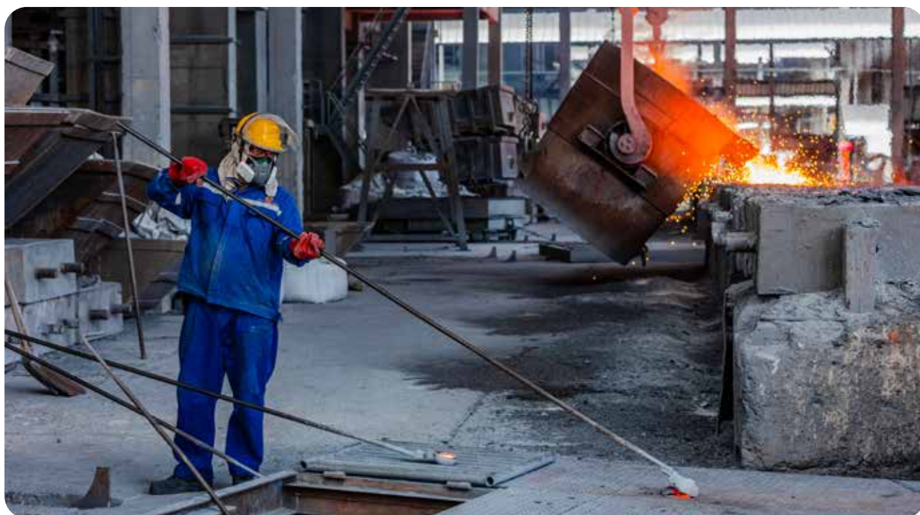
Worker at OM Sarawak takes product sample to be tested by soaking or splashing it with water.
